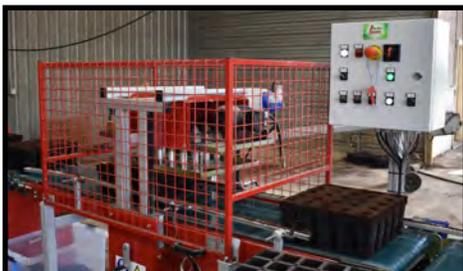
Next, a Pneumatic Dibbler creates the holes in which we will plant the seedlings. Further down the line, team members stand on either side of the conveyor and skillfully place plants until the container is full.
